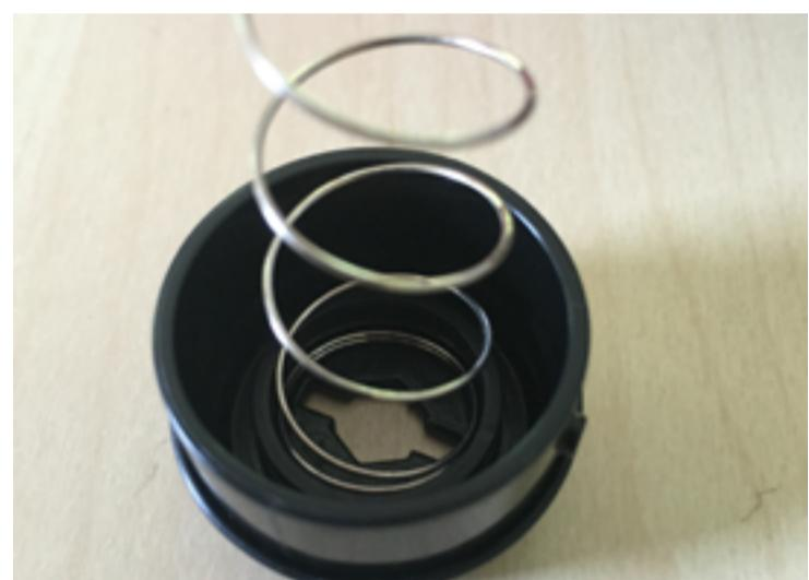
Look inside the bottom of the valve block – you will see the key cutout at the top end of the valve block.
