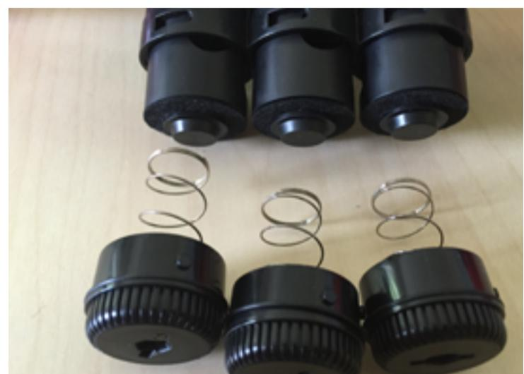
To replace the piston, place the spring into the bottom cap – the spring will fit snuggly inside the bottom cap center-ridge.
