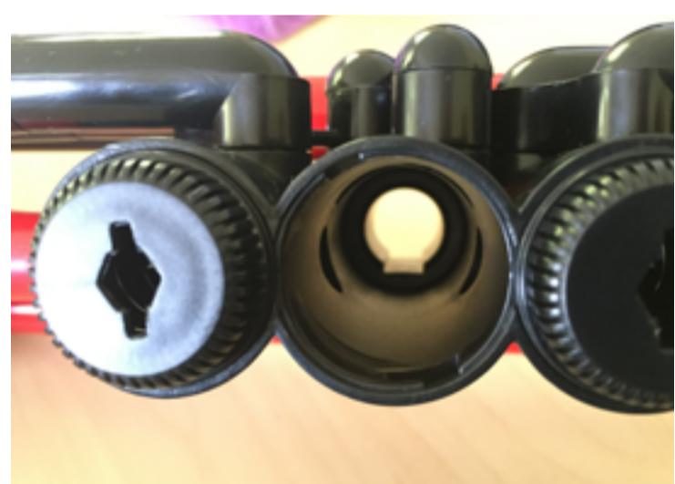
Finally, secure the valve bottom cap by pushing upwards into the bottom of the valve block and turning 10mm clockwise.
